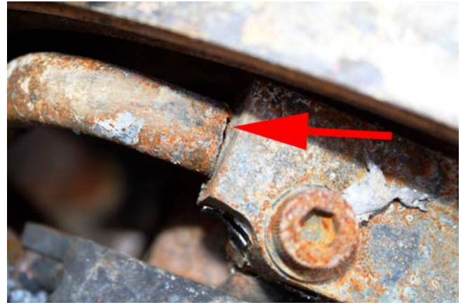
A cracked oil feed line to turbo was the cause
