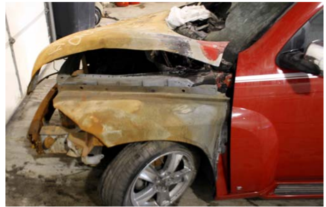
Fire started in front of the vehicle after it was turned off
