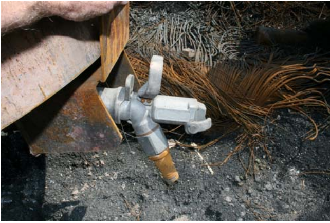
The above vehicle was totally destroyed as a result of a defective auto shutoff filler valve causing diesel to over fill the tank and the vehicle left running while being fueled
