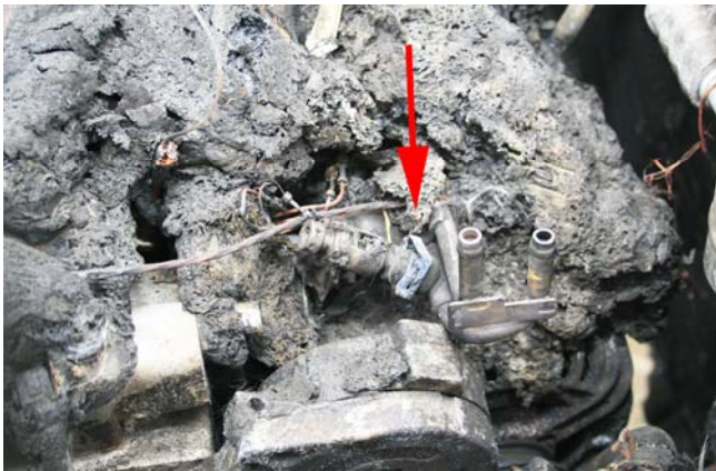
Improperly installed fuel injector destroyed this vehicle
